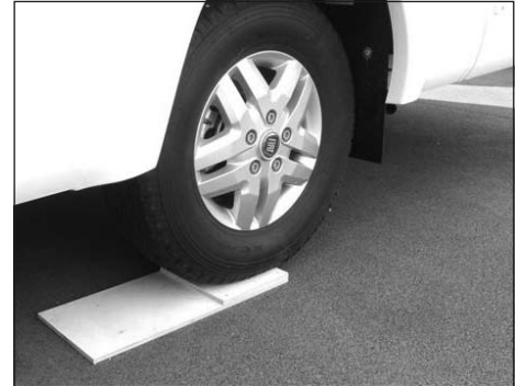
Fig. B Stepped levelling board
